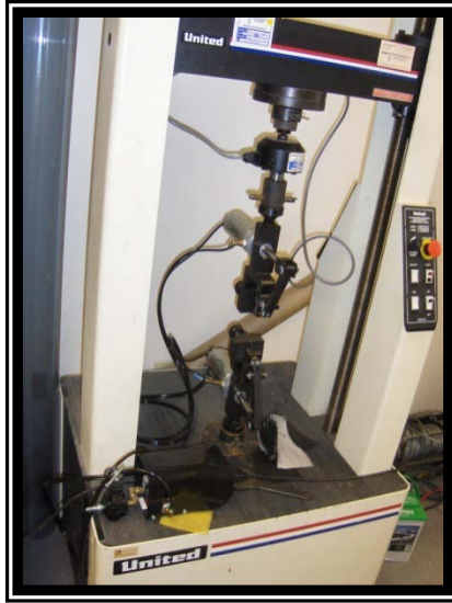
Figure 1 Apparatus for grab breaking load and elongation of geotextiles (tensile testing machine with quick release adapter and clamps) – ASTM D4632 and D5035
