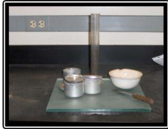
Figure 12 Apparatus for determining liquid limit and plastic limit of soil – ASTM D4318
