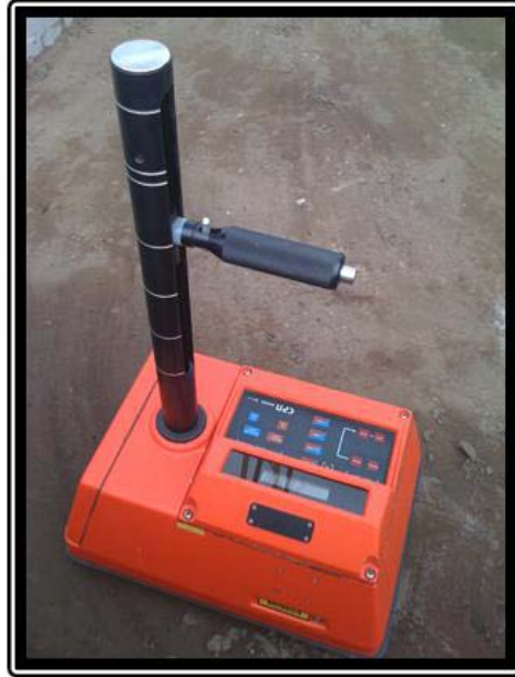
Figure 6 Apparatus for determining field moisture and density/unit weight by nuclear density gauge – ASTM D6938
