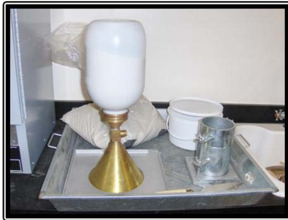
Figure 5 Apparatus for determining density/unit weight by sand cone method – ASTM D1556
