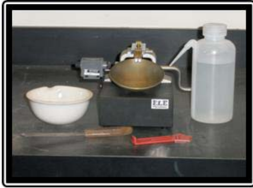
Figure 12 Apparatus for determining liquid limit and plastic limit of soil – ASTM D4318
