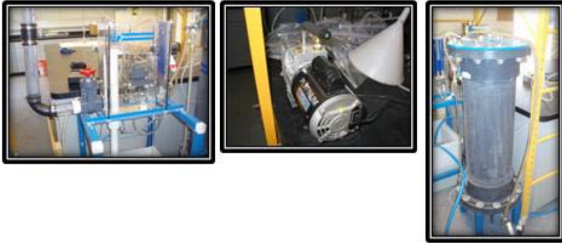
Figure 2 Apparatus for geotextile permittivity test (permittivity system, de-airing device and vacuum pump) – ASTM D4491
