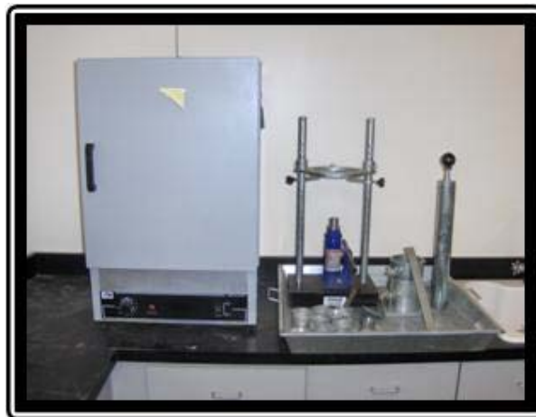
Figure 10 Apparatus used in compaction test – ASTM D698
