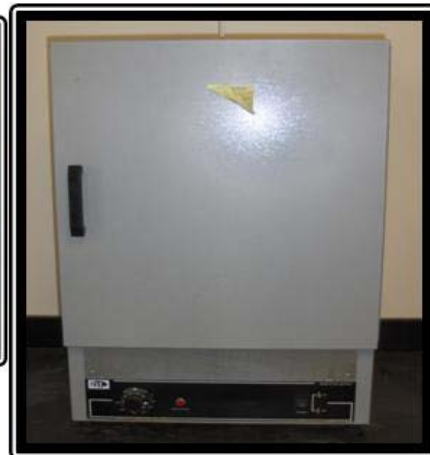
Figure 8 Apparatus for determining moisture content of soil – ASTM D2216 and D1140
