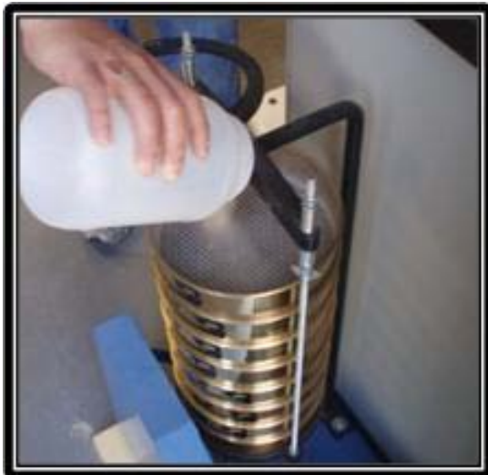
Figure 9 Apparatus for determining soil grain size analysis – ASTM D422
