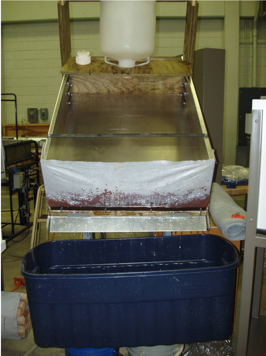
Figure 2 Experimental set up for flume testing.
