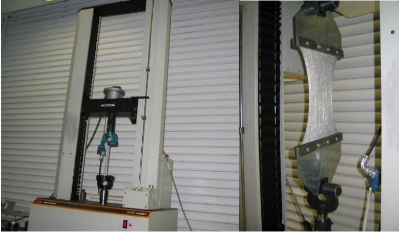
Figure 14 Testing apparatus and test specimen under load during the grab testing of BSRF fabric.
