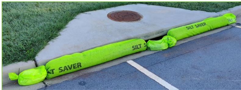
Use multiple SS 300s for large inlet openings Create adjustable weir with ends containing sand or stone bags.
